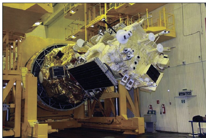
One of the Meteor M2 satellites undergoing testing prior to mating with its Fregat launcher Image: Roscosmos
