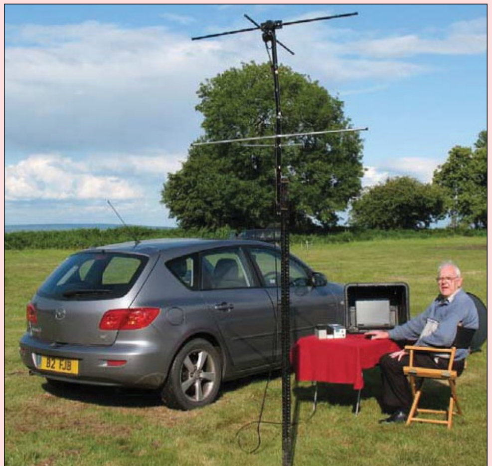
Almost everywhere he travelled, Francis delighted in taking his minimalist, portable APT kit with him, sometimes even resorting to the use of a simple antenna fashioned from a metal coat hanger. Here he is pictured on location with a turnstile antenna.
