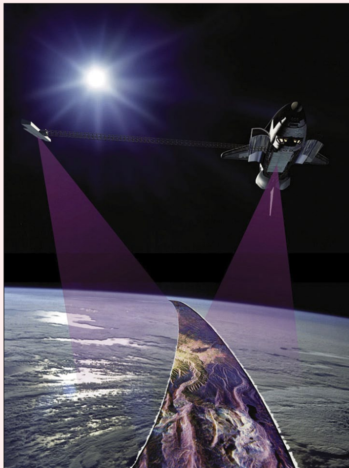
This artistic rendition shows Endeavour in orbit with the SRTM boom extended, while surveying Earth Image from the NASA image and video library
