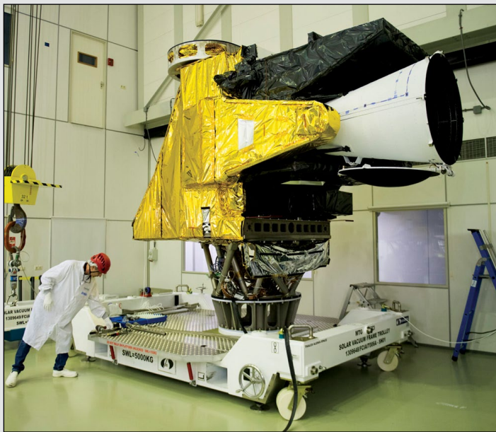
The Flexible Combined Imager unit undergoing testing Image: ESA
