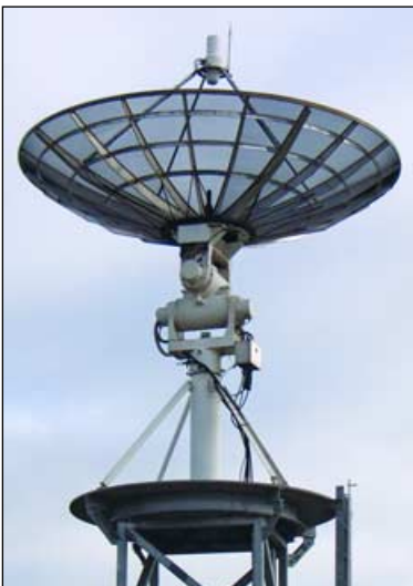
Figure 11 - XY-mount Polar Orbiter Antennas
