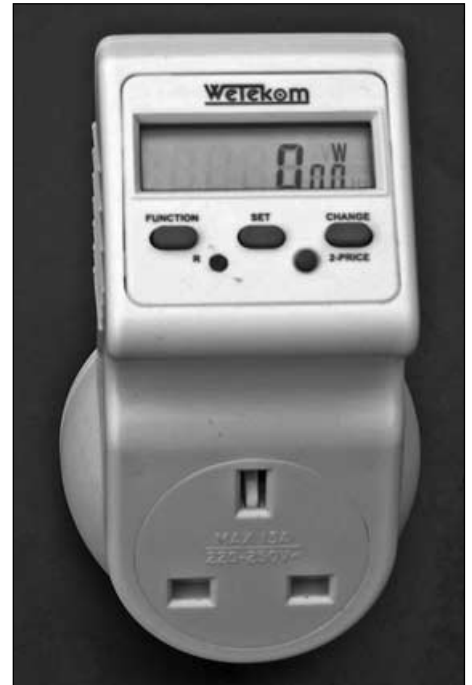
The plug-in-the-wall meter
