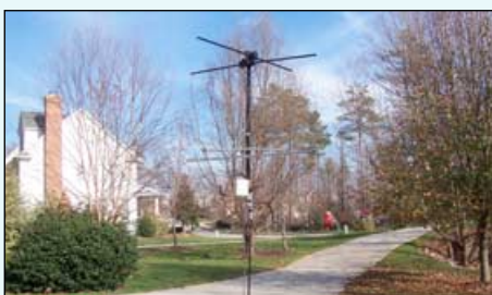
The reassembled turnstile antenna
