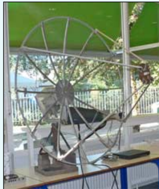
Figure 6 - X-Y drive antenna mount
