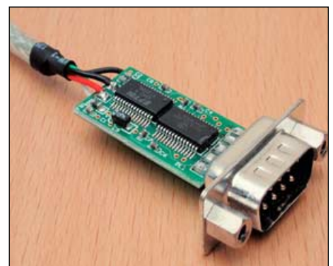
Figure 7 - A full-function USB converter
