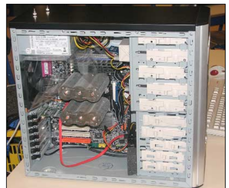
Figure 2 - Heat radiators inside Arne's PC
