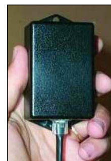
The small active direction-finding antenna used with LD-250, which is able to tell from which direction the signal is coming.
