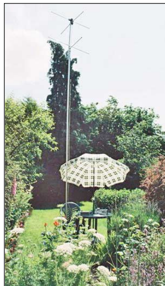
The pole-mounted turnstile
