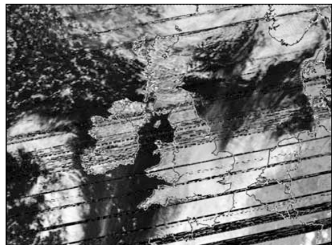
Figure 2 - Moderate pager interference present NOAA 18 channel-2 APT image at 13:24 UT on May 29, 2005, received on 137.91 MHz using the MSR50 receiver
