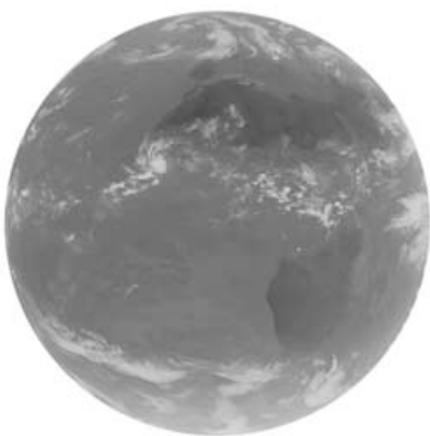
CHANNEL 11: Infrared 13.4 (12.4 - 14.4 \mu\text{m} )
