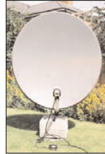
Photograph 6 Dish aligned on Astra at 19.2°E
