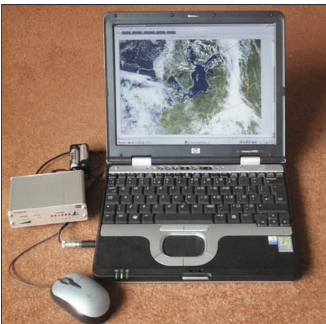
Figure 4 My mobile weather satellite ground station, consisting of the R2FX receiver with 4 x AA battery pack and notebook PC.
