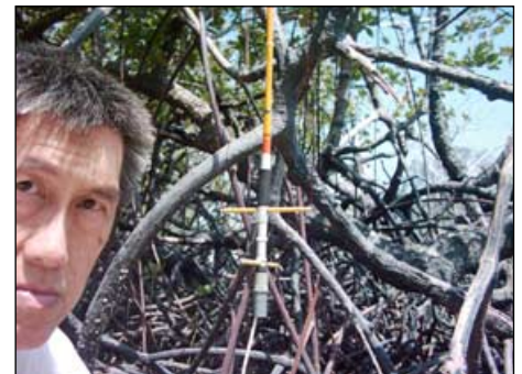
Figure 8 - C S Loh is a lecturer with Informatics in Kuala Lumpur. He is pictured above amidst mangroves, receiving wxsat signals with a home-made QFH built from SWG21 copper wire and a 1.8 metre glassfibre fishing rod—the CAST (Compact Antenna for Satellite Tracking). The antenna is connected to an RX2 receiver operated from a 9-volt battery and enclosed within a video-cassette holder: the CLEAR (Compact Light-mobile Experimental APT Receiving) system.
