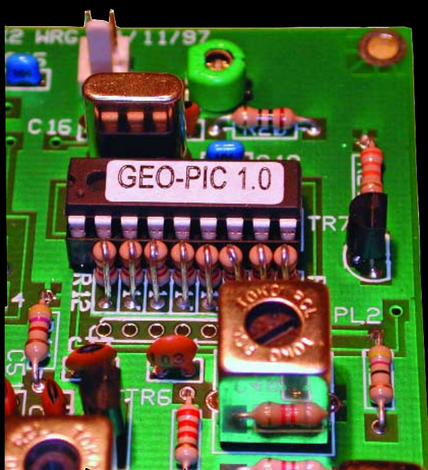
The main board of the RX2 receiver showing the new PIC in place at upper right.
