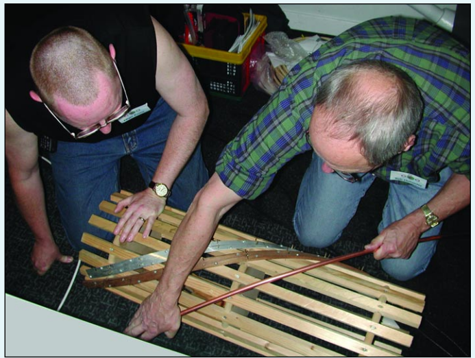
Nigel Evans and Rob Hollander (right) bending RQHF filars Photo: Cecilia Taylor
