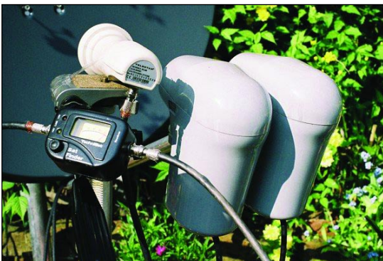
Figure 2 - Lining up the LNB with a Technisat 'Satfinder' meter
