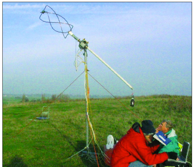
Figure 11 - The RQHA-12 under test (notice the weight to balance the set-up)
