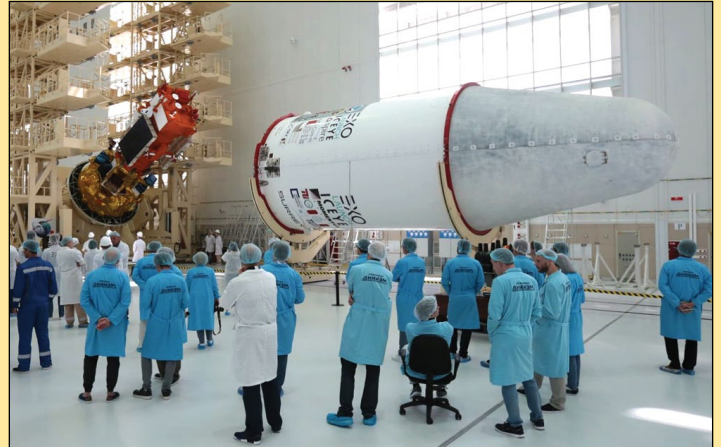
Personnel look on as the Meteor M2-2 payload is integrated with the Fregat-M upper stage of the launcher. Image: Roscosmos
