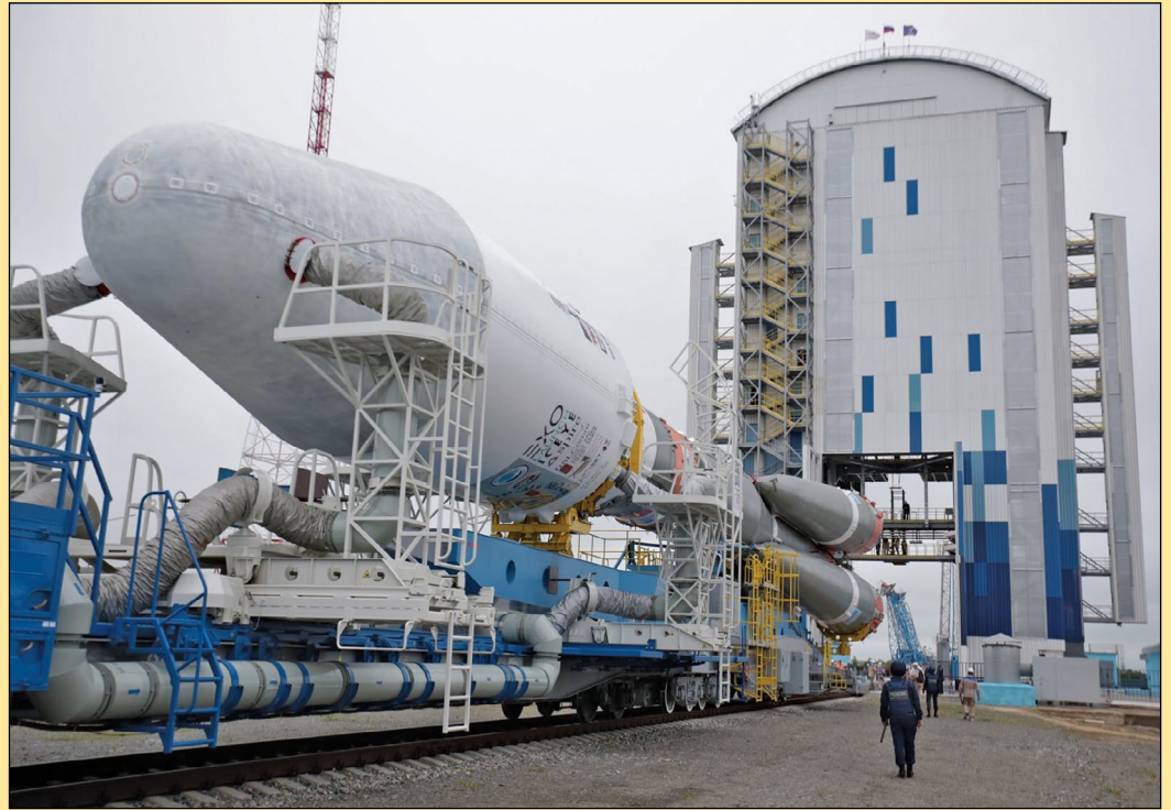
The Soyuz-2-1b/Fregat-M rocket being transported to its launchpad at the Vostochny Cosmodrome. Image: Roscosmos
