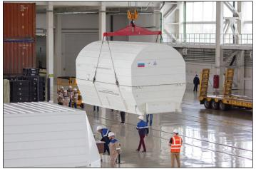
The upper stage of the Fregat launcher, which will carry Meteor M 2-2 into orbit, arriving at the Vostochny Space Centre for testing prior to the July 5 launch. Image: Roscosmos
