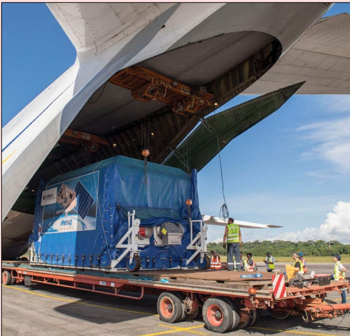
The Metop-C payload module is unloaded from the aeroplane's stern. Image: EUMETSAT
