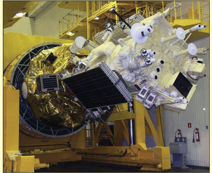
Meteor M2-1 undergoing leakproof testing prior to mating with the Fregat launcher Image: Roscosmos
