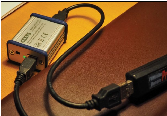
Improved reception is achieved using a USB isolator which contains an IC for galvanic separation
