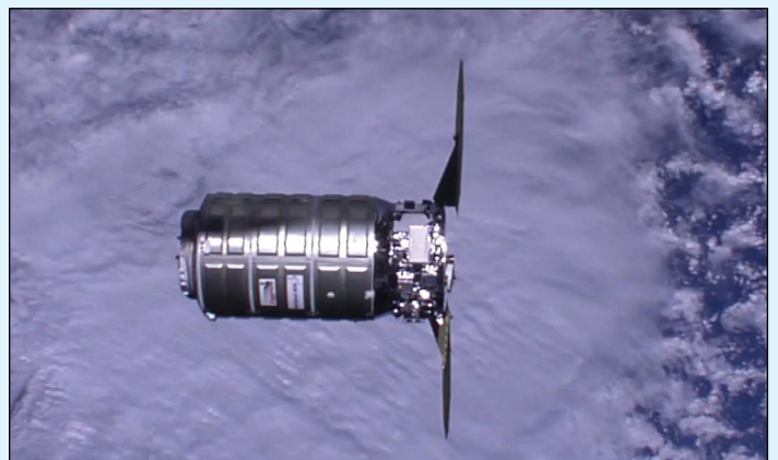
Figure 4 - The Cygnus module, caught by the HD TV Earth viewing camera. Comments from NASA ground control indicated the module to be about 100 m from the ISS. Rather surprisingly, the module's docking port seems to be located at the complex end of the module as seen on the left of the image.
