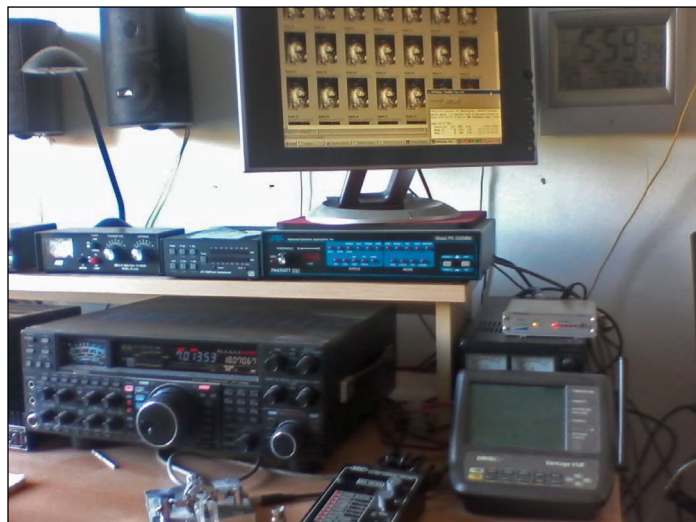
Figure 4 - FT-2000, Pakratt PK-232 tnc, R2ZX receiver and Davis Vantage VUE weather console
