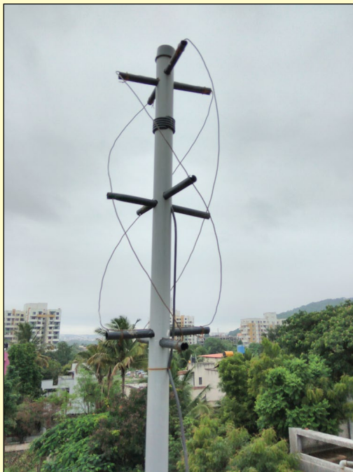
Figure 3 - The author's homebrew QFH antenna for NOAA reception
