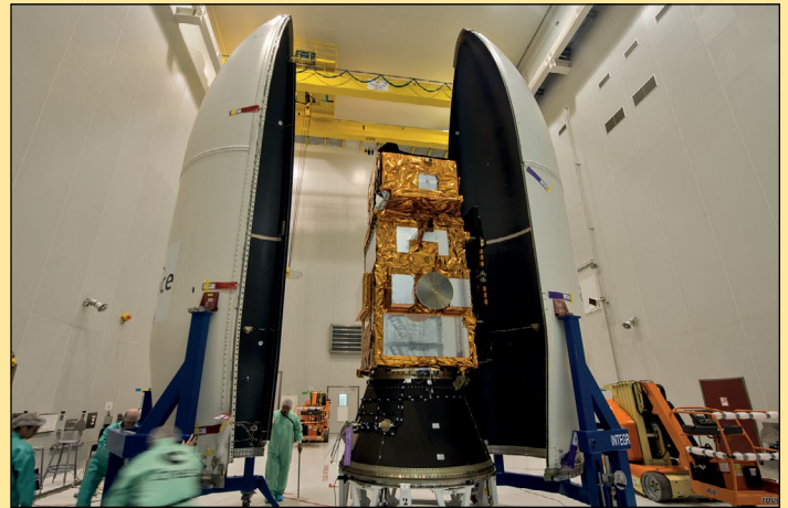
Sentinel-2A being encapsulated within the half-shells of the Vega rocket fairing, on 6 June 2015. Image © ESA / M Pedoussaut, 2015
