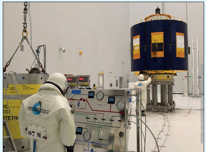
MSG-4's propulsion tanks are filled during launch preparations. Photo: ESA-CNES-ARIANESPACE
