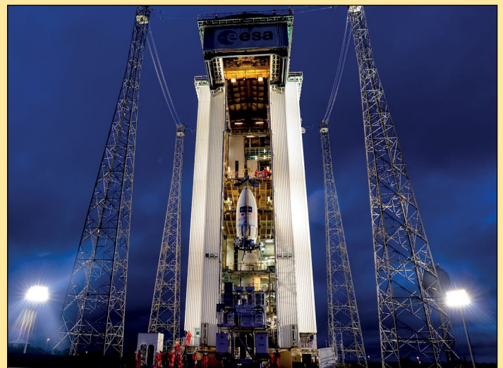
Integration of the fairing of Vega VV05, carrying Sentinel-2A, in the launcher assembly area at Kourou, French Guiana. Image © ESA / M Pedoussaut, 2015
