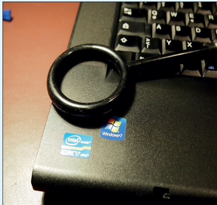
Figure 3 - Measuring magnetic near-fields on the laptop bezel.
