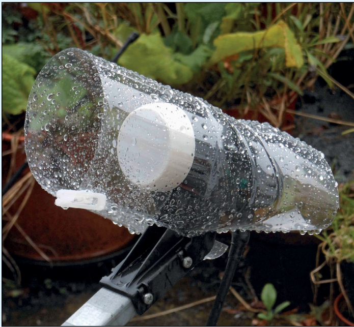
Figure 7 - A simple, but effective, LNB rain cover.
