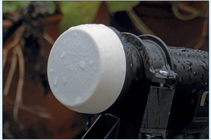
Figure 6 - Smaller raindrop accumulation causing minimal signal loss.
