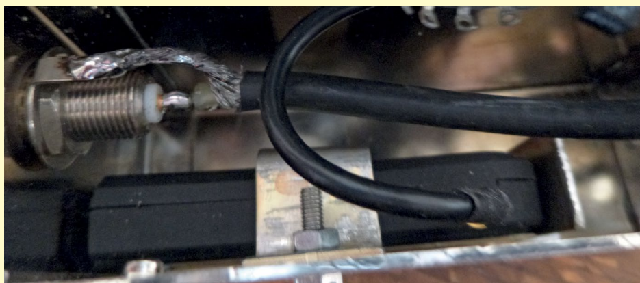
Figure 2 - A close-up photograph showing the dongle encapsulated in its metal box
