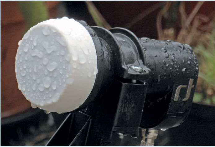
Figure 5 - Large raindrops on the LNB causing severe signal loss.
