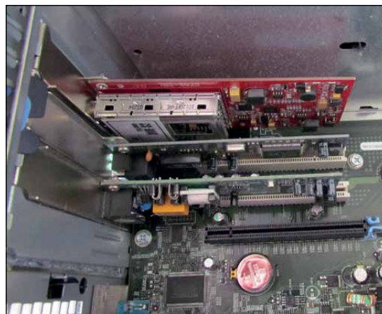
The illustration above shows the TBS-6925 card and the one below the unit installed into the PC.
