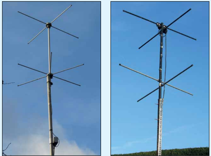
Figure 2 - The two antennas used by the author, with preamp (left) for the FUNcube Pro+ and without a preamp for the DVB-T+DAB+FM Dongle.
