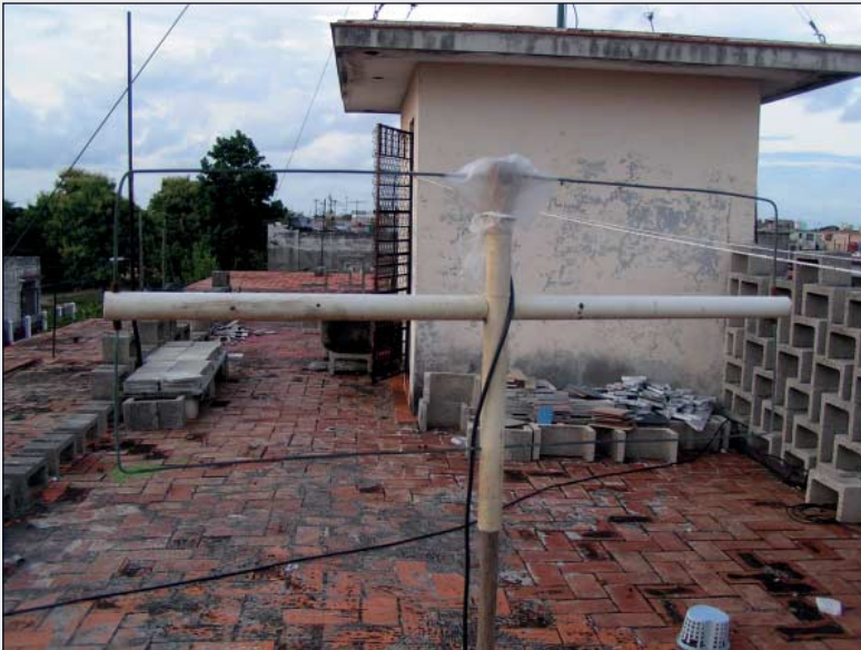
Figure 5 - The 'test' single Moxon is still in use three years after being built
