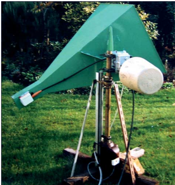
Figure 9 - The pyramidal horn antenna built by Les Currington
