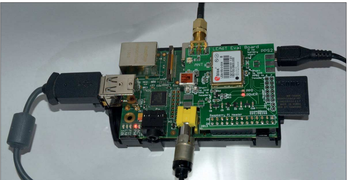
Figure 2 - The Raspberry Pi Computer with a GPS Module attached
