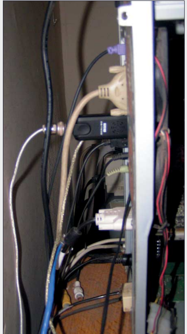
Figure 7 The RTL-SDR EzTV645 dongle and FC0013 tuner attached to the rear USB ports of the author's computer.
