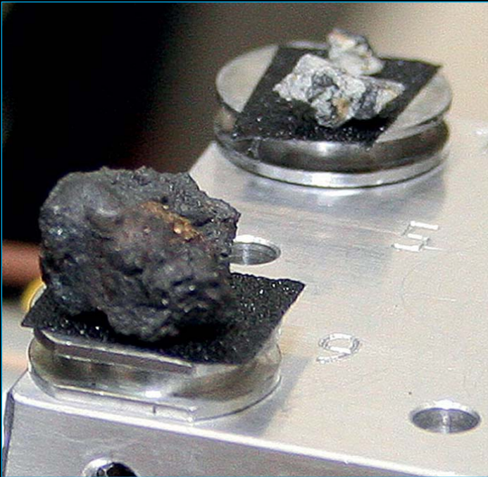
Figure 16 - Pieces of the Chelyabinsk meteor seen in a laboratory in Yekaterinburg. Black shock veins are visible in the broken specimen in the background. Credit: The Urals Federal University Press Service / Alexander Khlopotov
