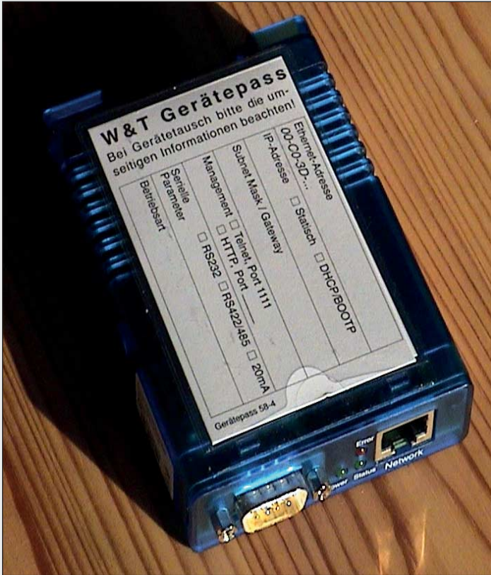
Figure 5 - The MiniIndustry 58211 COM server. The RS232 interface is to the left and the Ethernet-based network interface to the right.
