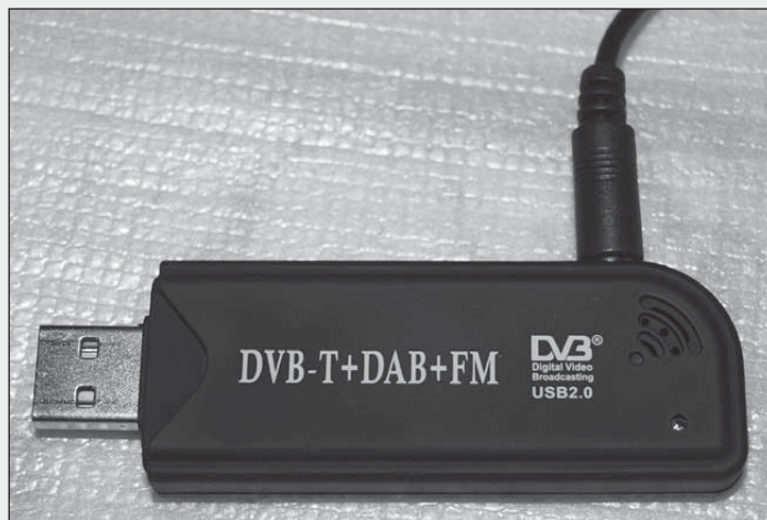
Figure 1 - This is the entire hardware part of the APT receiver.
