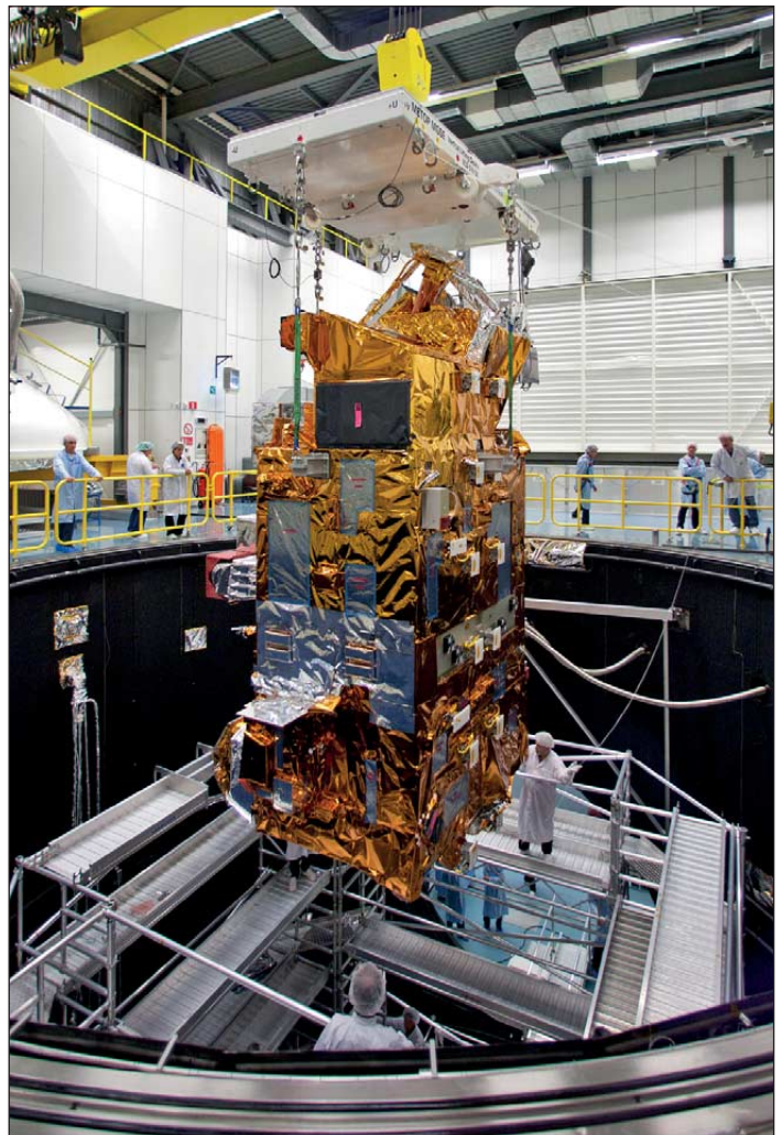
The Metop-B Payload Module is lifted out of ESTEC's Large Space Simulator, after more than a month of testing. Image: ESA
