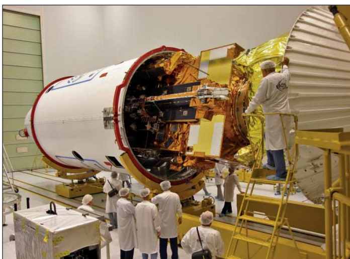
The Metop-B satellite disappears from view as it is eased into the rocket fairing in readiness for the launch on September 17, 2012. Image: ESA
