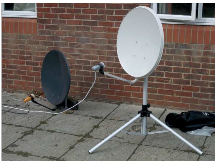
The Farnell tripod mounted 60 cm dish is shown on the right of this photograph with the author's fixed-mount 60 cm dish is on the left.
