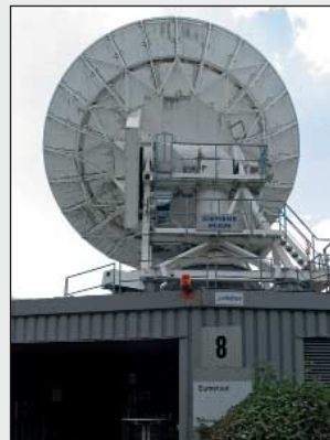
One of the EUMETSAT dishes with its control room at the base.
