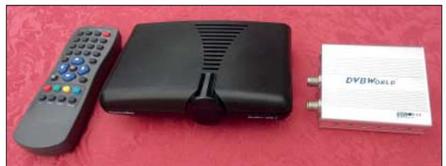
The popular DVBWorld receiver is shown here alongside the TechniSat USB 2 receiver (centre), now in service with GEO's mobile EUMETCast receiving station. Note that the remote control unit is not needed for EUMETCast reception but is useful if watching the many TV stations available on the same satellite's transponder.
