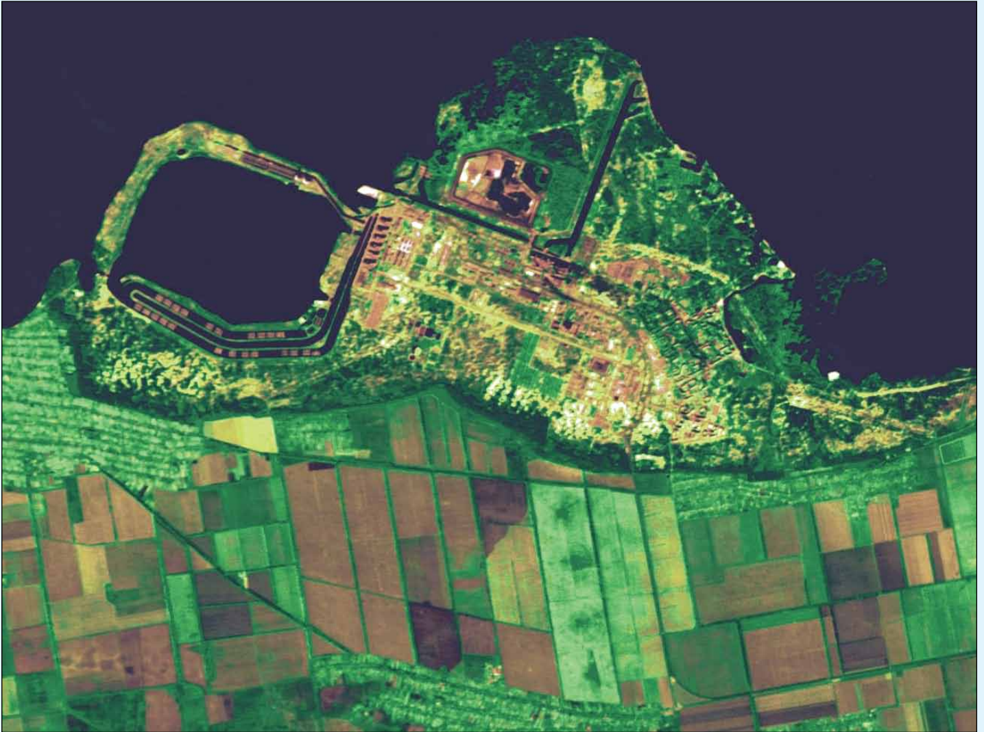
Figure 5 - Ukraine's new Sich-2 satellite took this 8-metre resolution image of Energodar on September 12, 2001, while undergoing initial testing. The large rectangular cooling pond adjacent to, and west of the Zaporizhzhya Nuclear Power Plant is hard to miss. The six nuclear reactor buildings can be seen, in a row, from the northeast corner of the pond. Image: State Space Agency of Ukraine (SSAU)
