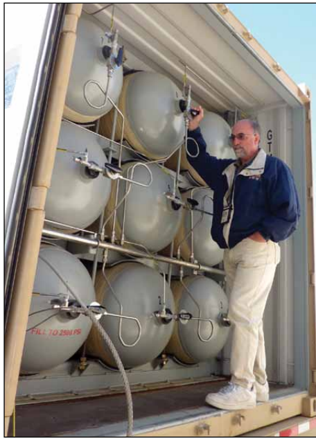
Tim Trenkle Backfilling Nitrogen Tanks
