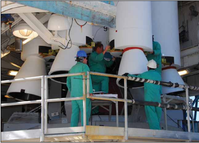
The 'business end' of the GEMs with a larger air ignited one to the left photo credit NASA/KSC
