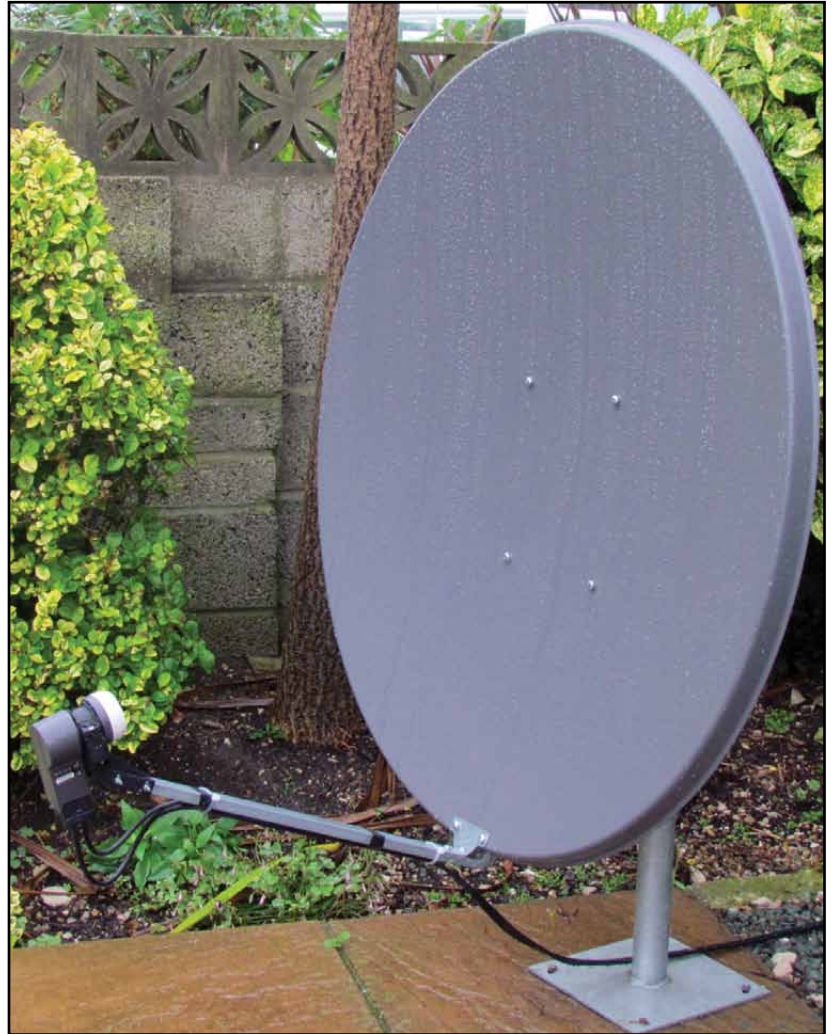
The author's 1-metre dish fitted with the twin LNB
