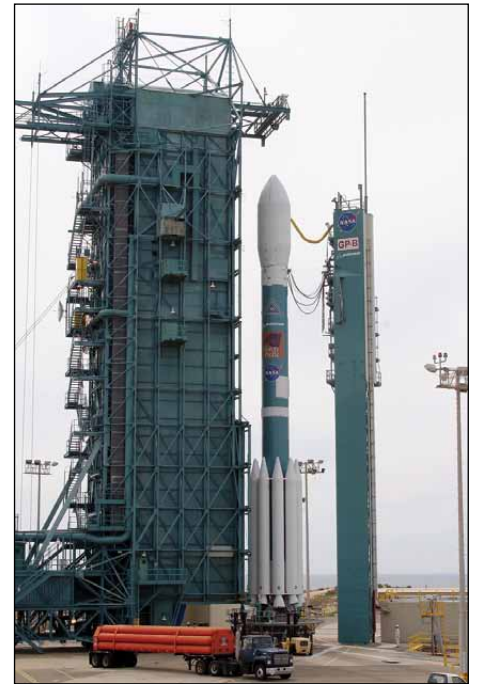
Gravity Probe B at SLC 2-W is a Delta II 7920-10. The mobile service tower is to the left and the fixed umbilical tower is to the right of the rocket. Credit: NASA/KSC
