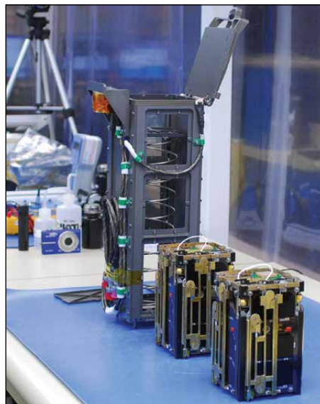
P-POD on the left and two cubesats on the right. Credit: NASA/KSC
