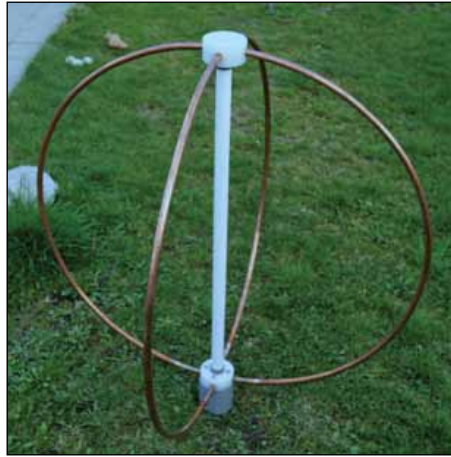
Figure 5 - Daniel Verschuieren's loop antenna
