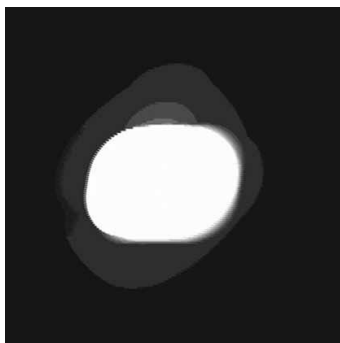
Figure 4 A straylight artifact on a Meteosat IR-3.9 image Image © EUMETSAT
