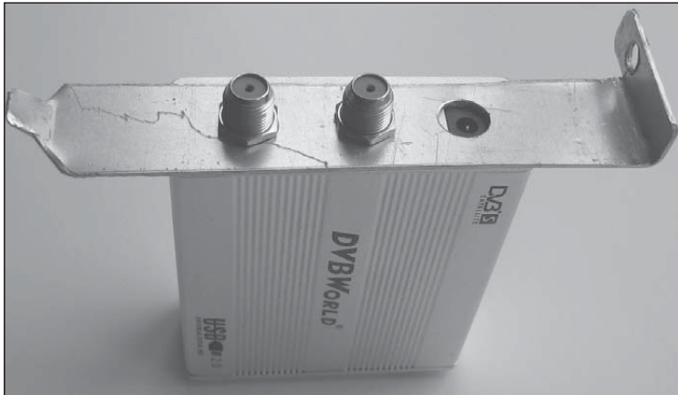
Skystar 2 internal card replaced by DVBWorld receiver fixed to new back plate
