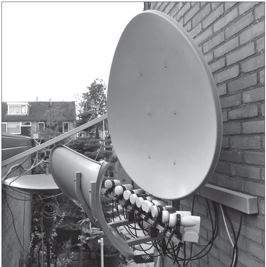
Figure 5 This single dish with multiple LNBS receives from satellites at 28.5°E, 23.5°E, 19.2°E, 16°E, 13°E, 10°E, 9°E, 5°E, 1°W and 5°W
