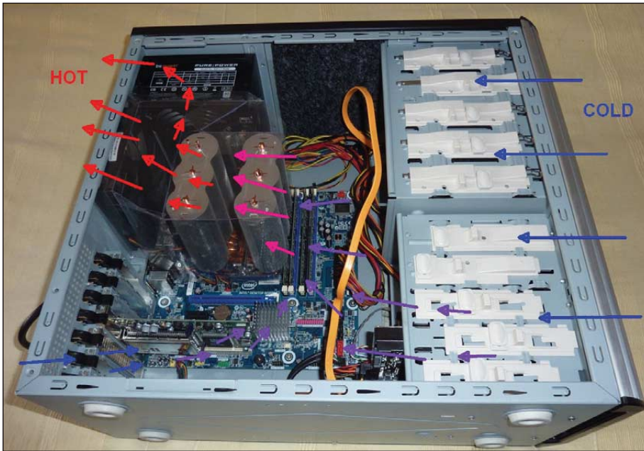
Figure 14 - PC with optimised cooling to provide low noise
