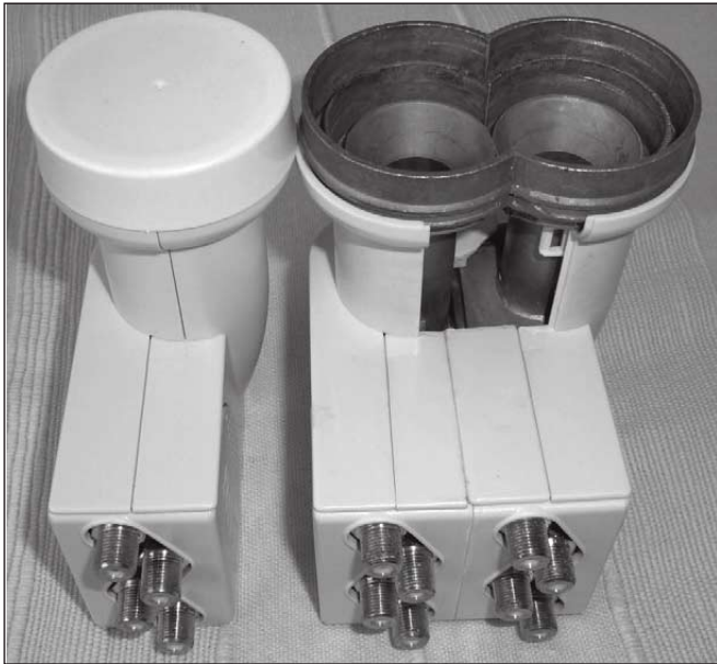
Figure 3 - The original LNB (left) compared with the 'TwinSat' LNB
