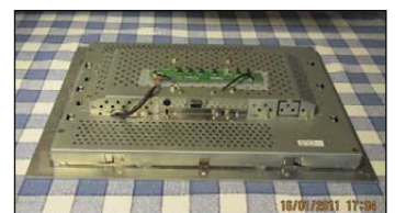
Figure 8 One element from the display unit (aluminum frame and screen element).
