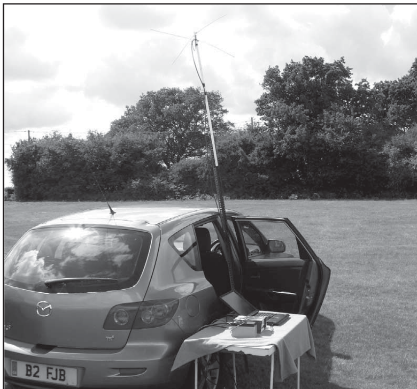
My APT station in the field. It consisted of my home built 137 MHz APT receiver which only consumes 100mA, my home made turnstile antenna and the power hungry laptop: all powered by the car battery.
