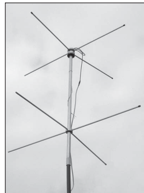
Figure 2 - A turnstile antenna
