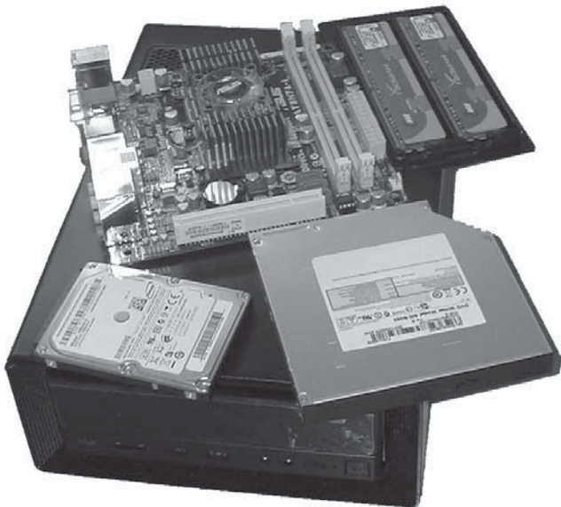
Figure 1 - The motherboard, hard drive and optical drive
