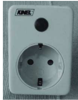
A simple mains-only SPD with fault indicator
