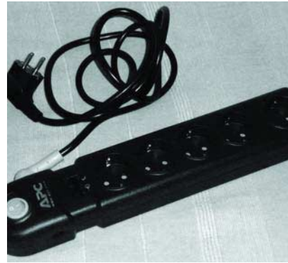
An SPD from APC protecting Mains and phone line, fault and earth indicator lights
