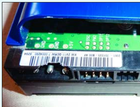
Close-up showing the damaged SATA socket Photo: Arne van Belle
