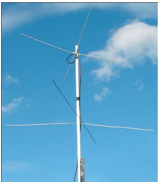
The coat hanger wire turnstile
