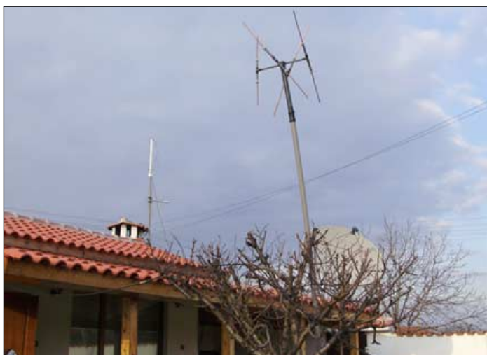
This photograph clearly shows the QFH and DCA on the author's roof
