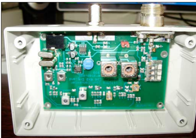
Figure 6 - A WEFAX Downconverter
