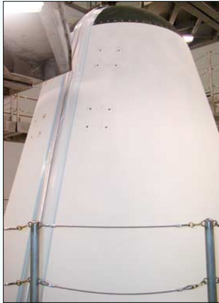
The fairing, showing tape running down its side. Explosive charges to release the fairing lie beneath this tape.
