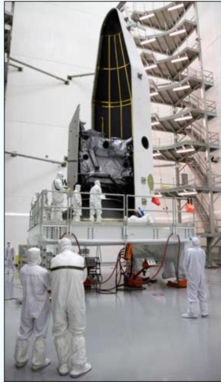
Encapsulating GOES-O Image: NASA
