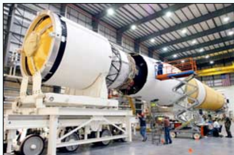
Mating the GOES-O Delta-IV 2nd stage to CBC Image: NASA
