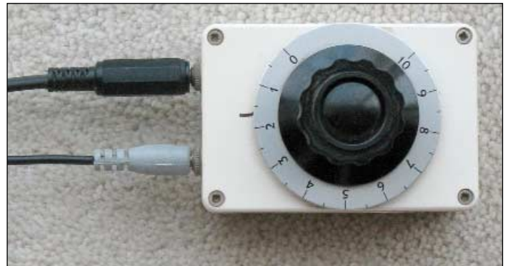
Figure 1 - The boxed and labelled potentiometer
