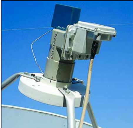
Figure 2 The LNB should be shifted up and down to fine tune the focal length. Please note the marks on the LNB, made for future reference using a waterproof marker
