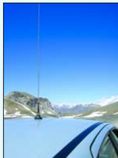
The whip antenna used to receive NOAA-15
