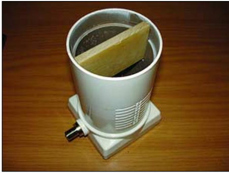
Figure 1 Make sure that the 'biscuit' is properly installed inside the LNB
