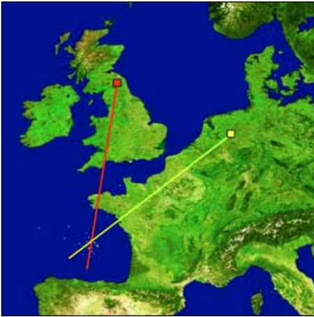
Figure 2 - Lightning Location by Triangulation
