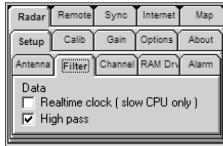
Figure 21 - Selecting a high-pass filter, which helps to eliminate spurious sources
